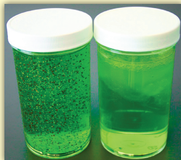
0.05% AxCel CG PX (no separation/uniform suspension) 0.25% Xanthan Gum (phase separation/product failure) In a high-surfactant body wash
