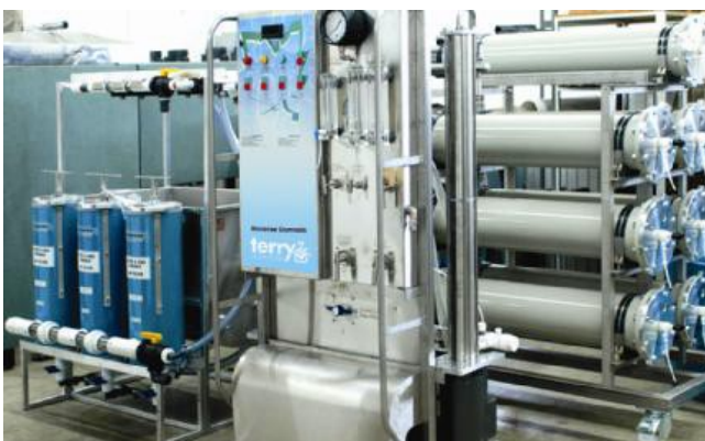
Reverse osmosis equipment for gentle concentration of the Aloe Vera gel
