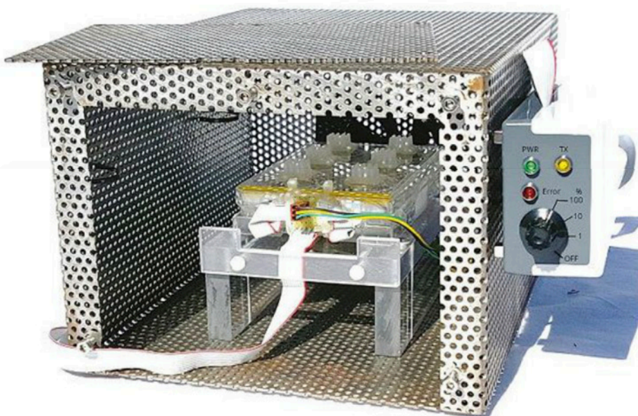
Figure 7: Cell culture WiFi emitter system within a Faraday cage.
